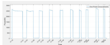
The power consumption curve of the oven for cooking at 180 °C temperature.
